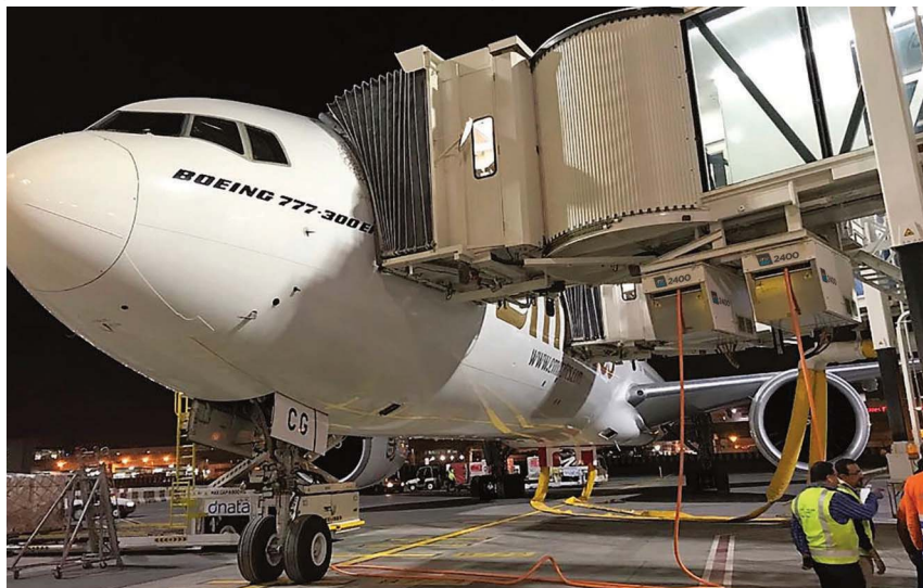
Helping the planet: Electrical power from ITW GSE bridge-mounted GPUs help reduce Dubai International Airport's carbon footprint.
