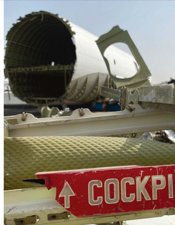
Valuable: Materials can be extracted from aircraft, such as this MD-11 currently being dismantled and recycled.
